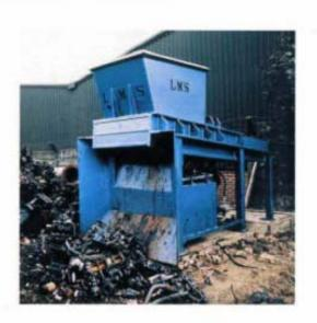
Both Engine Crushers have been designed and developed to meet the exacting standards required in the Scrap Industry and have replaceable wear plates for convenience. A wide variety of optional equipment is available on request.
