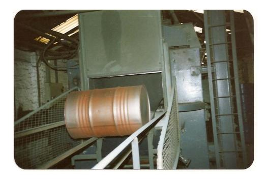
The Challenger Drumtech Airless Shot Blast Machine is fully automatic and will process 100 drums per hour dependent on the surface finish required. The machine does not use compressed air in the blasting process with the shot being recirculated via a feed screw from the base of the machine and a bucket elevator to the distribution hopper above the shot cabinet.
