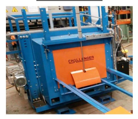
The Challenger Drumtech Automatic Air De-denter is designed to de-dent standard 205 litre capacity steel drums.
