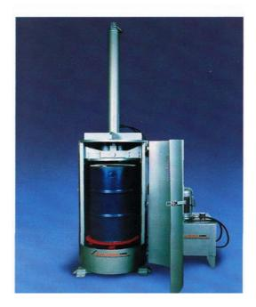
The Challenger Drumtech Drum Crusher has been designed to crush un-useable 205 litre capacity steel drums to a fraction of their original height to keep both site storage and transportation costs to a minimum.
