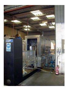
The Challenger Drumtech Drum Pre-Washer is designed to wash drums, kegs and other similar containers internally to remove the more difficult residues before going into the main Washer.
