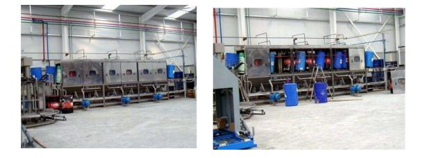
The Challenger Drumtech Drum and Cask Washer is designed to wash drums, kegs and other similar containers both internally and externally. Drums are fed into the machine by hand onto specially designed carriers, the start button is depressed and the machine proceeds through its washing cycle automatically.
