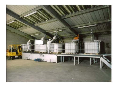
The Challenger Drumtech IBC Reprocessing Line is designed to wash, rinse and dry used IBC containers for re - use as a usable package generally as shown in the photograph above and the containers are transferred between stations by hand.
