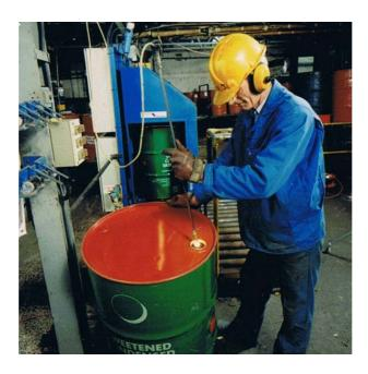
The Challenger Drumtech Inspection / Grading Station is designed to allow operators to visually inspect the inside of standard 205-litre steel drums to check for signs of corrosion and to determine each drums' suitability for grading purposes.
