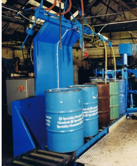
The Challenger Drumtec Steam / Vacuum Dryer is designed to give a controlled internal drying treatment in order to ensure optimum dryness inside the drum.
