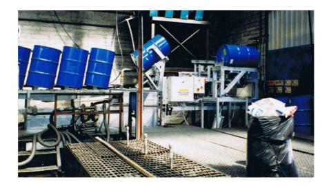
The Challenger Drumtech Automatic Loader is designed to automatically load standard 205-litre capacity steel or plastic drums into either a Pre-Washer or the main line Washer.
