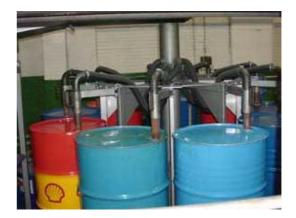
The Challenger Drumtech Carousel Hot Air Dryer is designed to give a controlled internal hot air drying treatment in order to ensure optimum dryness inside the drum.
