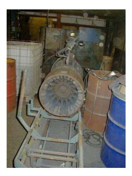
The Challenger Drumtech Expander can be used either alone as a semi or in a production line as a fully automatic machine.
