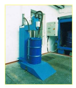
The Challenger Drumtech Recirculating Water De-Denter is simple to operate and will reshape badly damaged drums under hydraulic pressure. It allows all round accessibility to enable creases to be beaten out using leather mallets and it will process drums that will not generally seal on air type machines.
