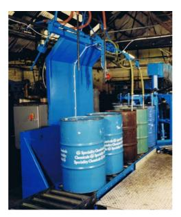
The Challenger Drumtech Carousel Hot Air Dryer is designed to give a controlled internal hot air drying treatment in order to ensure optimum dryness inside the drum.
