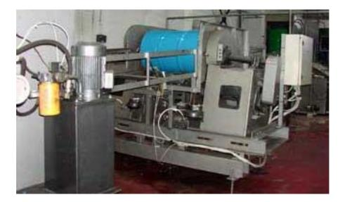
The Challenger Drumtech Automatic Double ended Chimber is designed to reform and seal chimbs of standard 205 litre capacity steel drums.
