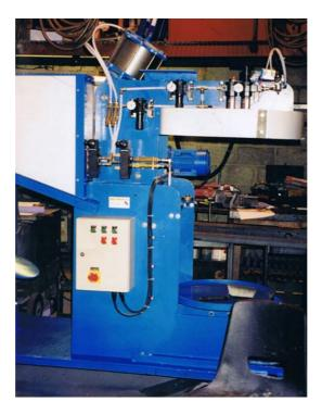
The Challenger Drumtech Cutter and Beading machine allows drums, which may otherwise be discarded due to leaks or for other reasons, to be converted into open top drums. One side is equipped with an efficient powered rotating cutting blade and on the opposite side is a beading system, which forms a safe edge to the cut end.
