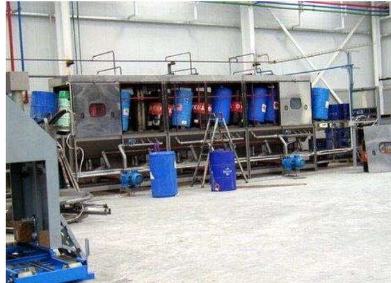
The Challenger Drumtech Drum and Cask Washer is designed to wash drums, kegs and other similar containers both internally and externally. Drums are fed into the machine by hand onto specially designed carriers, the start button is depressed and the machine proceeds through its washing cycle automatically.
