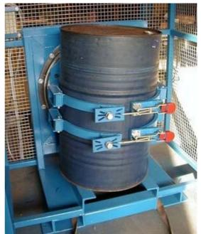
The Challenger Drumtech Drum Rotator / Mixer is designed to handle full 210 litre steel drums whereby the drum is securely clamped in place within a fully guarded enclosure and is rotated end over end in order to mix the contents.
