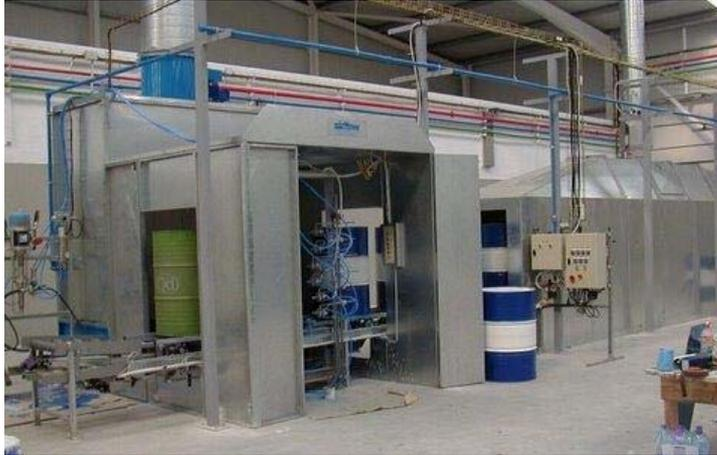
The Challenger Drumtech Drying Tunnel is fully automatic and has been designed to be sited in a Drum Reconditioning Line immediately after the Automatic Paint Station to dry the recently painted drums before other operations take place.
