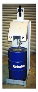
The Challenger Drumtech Semi Automatic Leak Detector will handle standard 205 litre capacity steel or plastic closed top drums, which are clean and dry in line with International quality control requirements.
