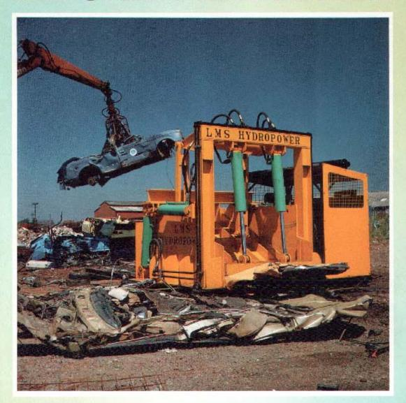
The LMS Car Flattener is one of the most interesting Flatteners on the market. Fitted with the latest PLC Controller, which eliminates all electrical Limit Switches, preventing minimum stoppage of production. It also ensures that under no circumstances can this Flattener become overloaded.
