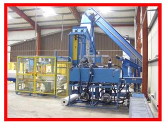
The Challenger Mass Measuring Baler has been developed to weigh, compress and balea variety of baled materials such as chopped hay, chopped straw, shredded paper, woodchips, woodshavings, etc. They can be manufactured to a wide variety of specifications to manufacture bales with a mass of between 1 kg and 25 kg and can produce bales at a rate of up to 400 bales per hour.
